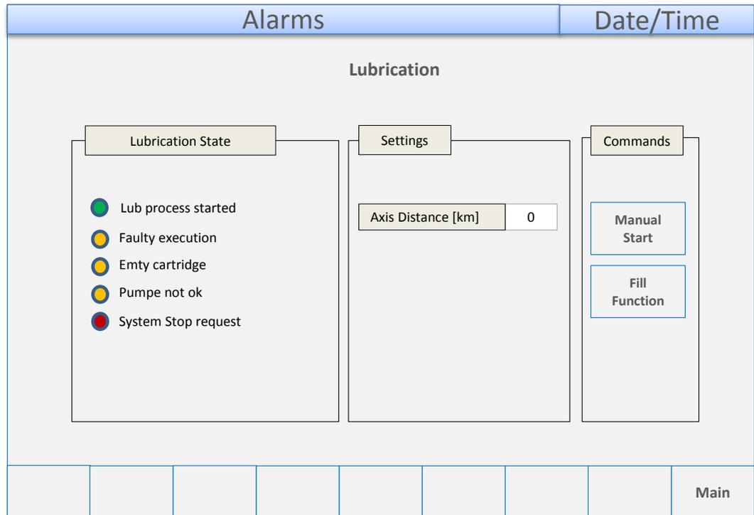
Fig. 8 Sample HMI page with minimal implementation
