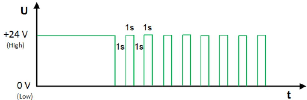
Fig. 6 Timing diagram for empty cartridge
