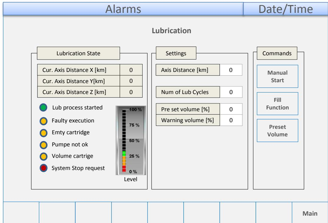
Fig. 9 Sample HMI page with maximal implementation
