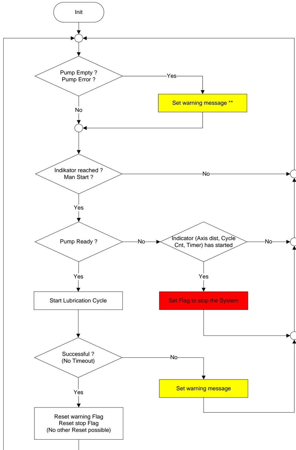
Pump Ready = No Error (5s Input) **AND** Not Empty **AND** Lubrication process not started
