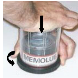
2. To open, place the lubricator on a flat surface. Press the hood downward and turn the black ring counterclockwise.
