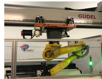
Güdel TrackMotion Overhead (TMO) carrying FANUC M20iA/35M robot
