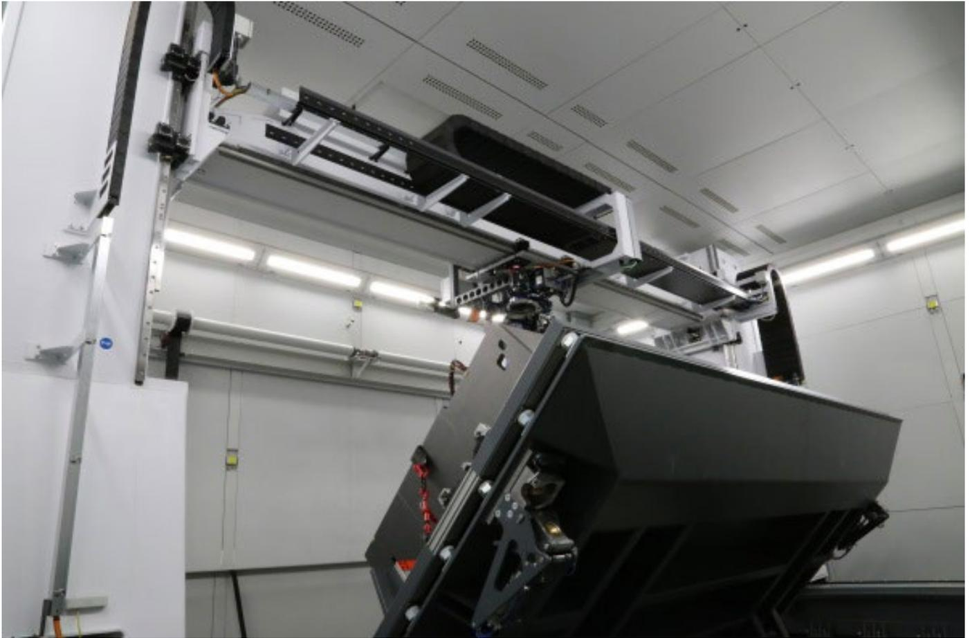
drive (master) controls the second (slave). High-precision planetary gearboxes from Güdel are used in all axes. The planetary gearboxes are characterized by high rigidity and power density, and ensure there is additional reliability in the application results. Güdel's roboMover gantry system permits effective strokes of 4.6 x 6.1 and 1.85 meters.
