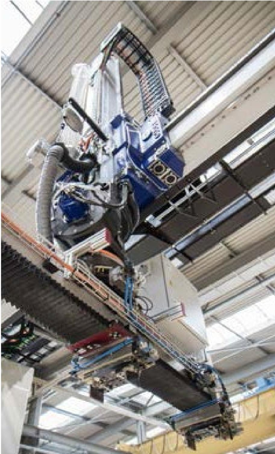
The gantry robot for wood processing at Erne moves along a stretch of over 50 meters. For even more efficiency, it carries its tool magazine and two spindles with it. The tool change between the gripper and saw is carried out smoothly. Waste, such as splinters and dust, is disposed of using an automatic extractor in the container provided. The change/calibration stations are positioned directly opposite the two system operators for optimum visibility.
