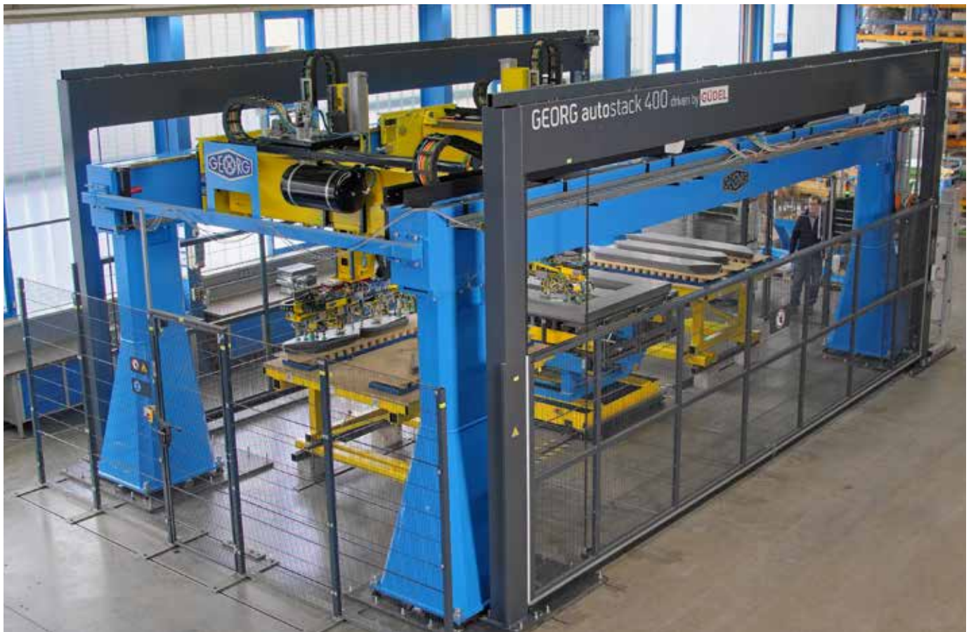
GEORG autostack 400, driven by Güdel (offline core stacking solution for distribution transformer cores)
