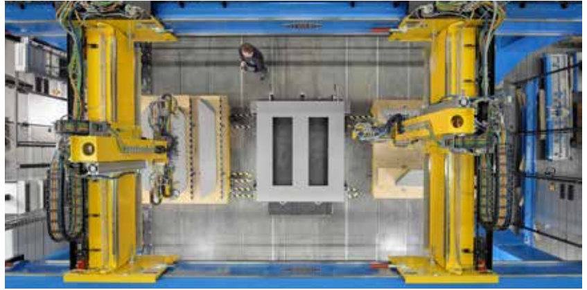
GEORG autostack 400, driven by Güdel (offline core stacking solution for distribution transformer cores)
