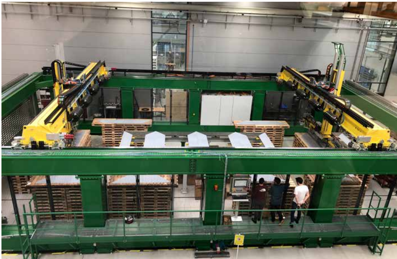
GEORG autostack 1000, driven by Güdel, currently under production (offline core stacking solution for transformer cores up to 5 limbs with yoke length up to 9 m)
