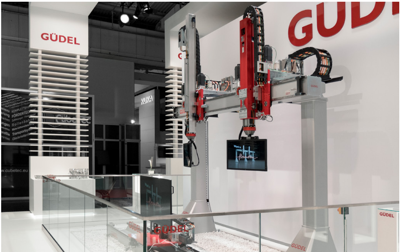
The new telescopic axis (right) with the same performance features as the fixed axis (left)
